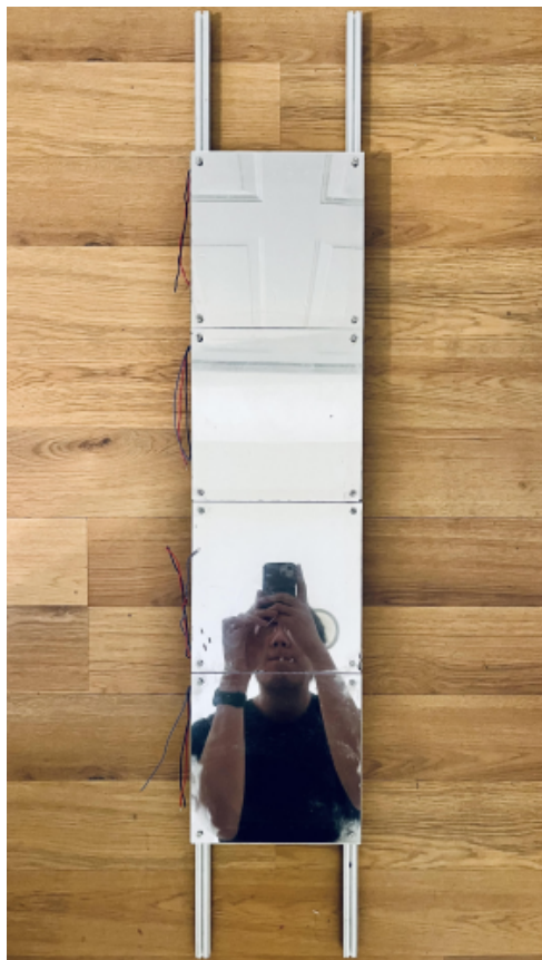
Figure 2 (left): An initial prototype of the panel attachment mechanism (as partial structure) completed in 2017. The four corners are attached with little machine screws that can be slid into the maker beam.
